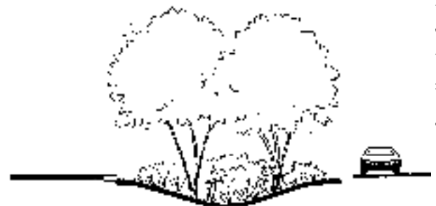
Cul-de-sac infiltration island accepts stormwater from surrounding pavement. Note flat curb.
