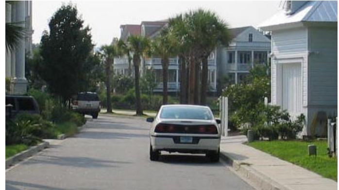
Mt. Pleasant, SC: An 18 foot wide street can accommodate parking on one side of the street. Streets as narrow as 22 to 24 feet wide can accommodate parking on both sides if parking is not frequent.
