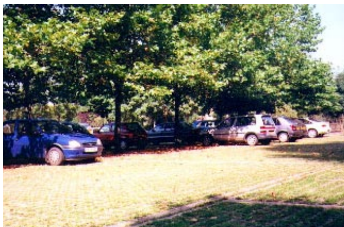
A parking lot with Grasscrete™ interlocking pavers. Bordered by a stream and with no option for piped drainage, this university parking lot has been draining naturally for 20 years.
