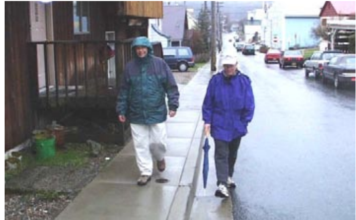
A narrow sidewalk – 4 feet or less in this case – may not provide enough space for two adults to comfortably walk side by side.
