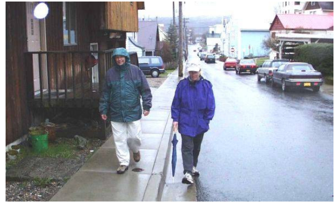
A narrow sidewalk – four feet or less in this case – does not typically provide enough space for two adults to comfortably walk side by side (location unknown). Source: Michael Ronkin
