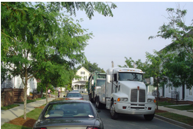
A 20-foot wide street with parking on one side does not compromise access by emergency responders or other large vehicles (Huntersville, NC). Source: Tom Low, DPZ
