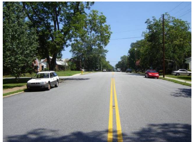
An example of a collector street that has infrequent on-street parking and too much pavement, which likely encourages speeding (Westminster, SC). Source: Upstate Forever
