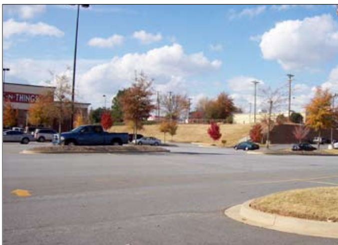
While increased parking lot landscaping provides many benefits, the curbed islands result in limited storm water retention potential (Spartanburg County, SC).
