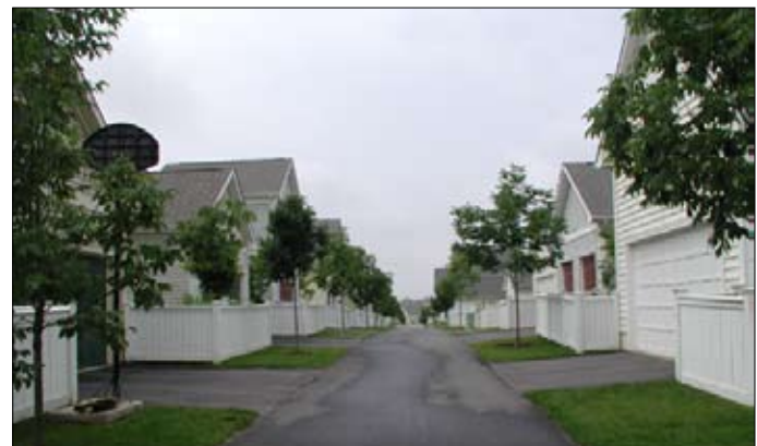
A 12-foot alley with trees and no curbs serves houses on approximately 40-foot wide lots (Gaithersburg, MD).
