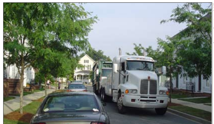
A 20-foot wide street with parking on one side does not compromise access by emergency responders or other large vehicles (Huntersville, NC).
