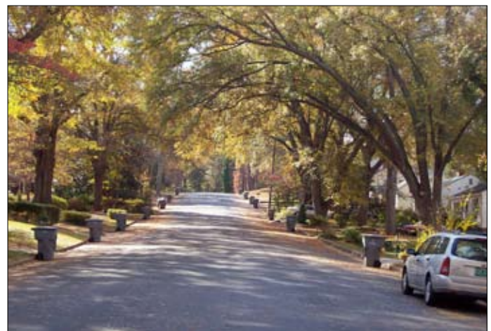
An example of a collector street that has infrequent on-street parking and too much pavement, which likely encourages speeding (Spartanburg County, SC).
