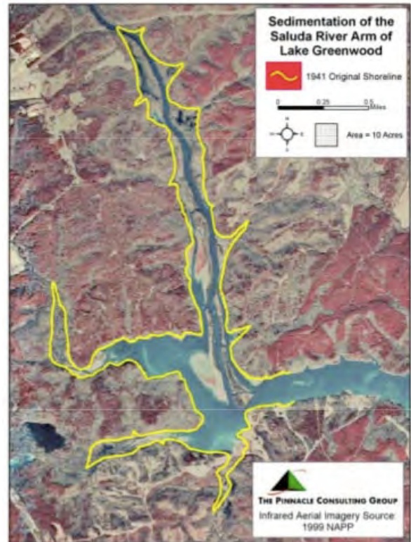
This aerial photo of the Saluda arm of Lake Greenwood shows how much of the lake's original area has been lost to sediment.
